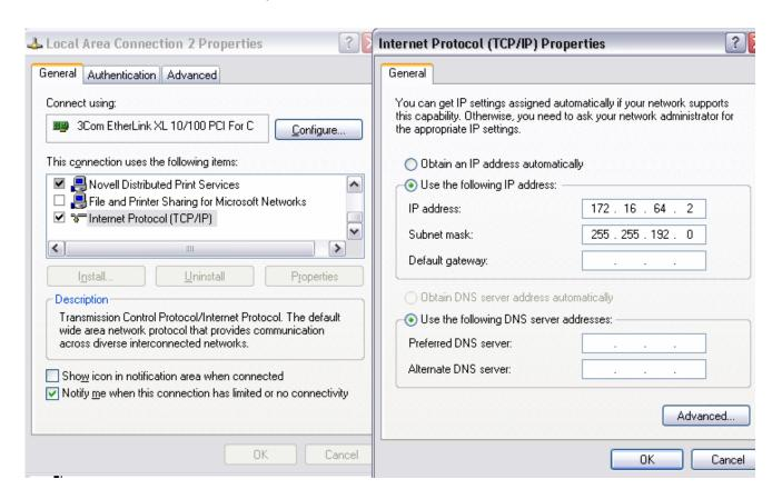
Note that the IP Address and Subnet Mast must be the same as set in T-PDS & the GEN651A (the last digit of the IP Address must be different however, it cannot be .1 The address of the GEN651A module is 172. 16.64.1). Click OK. In case of difficulty setting up the computer Ethernet card, contact the company MIS/IT Department.
